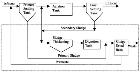
Figure 1. Conventional activated sludge treatment facility
